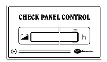
CRSC-07 indicator has been designed to control power batteries for electric vehicles and can be used to monitor stationary batteries used to supply board equipment on mobile vehicles. Including the hour meter, it can indicate operating time and is therefore very useful for maintenance programs.
