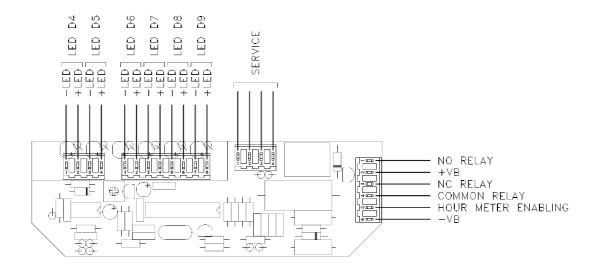
\* To enable counting connect the input (PIN5) to battery positive
